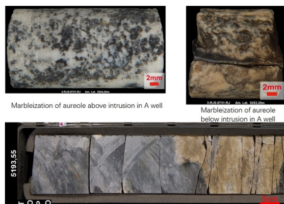
Fig. 1 – Marbleization of the intrusion aureole in pre-salt limestone in the Libra Area, Santos Basin.
